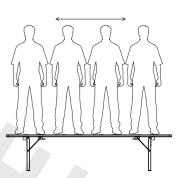
In the FE analysis, the previous underframe was compared with the new underframe. The table or bench legs were clamped tightly for this purpose at the top and at the snapper. A force F acts from the outside at the bottom. This calculation method simulates swaying in the longitudinal direction.
